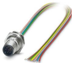
Device connector rear mounting, Universal, 12-position, Pin, straight, M12-SPEEDCON, A-coding, on free cable end, Individual wires, cable length: 1 m, 0.14 mm<sup>2</sup>, TPE litz wire, potted, this item is expected to be lead-free from Q2 2026 in accordance with RoHS II without exception 6c (Pb < 0.1%), a lead-free alternative is possible on request in advance
