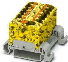
Distribution block, nom. voltage: 800 V, nominal current: 32 A, number of connections: 13, connection method: Push-in connection, Rated cross section: 4 mm<sup>2</sup>, Load contact, cross section: 0.2 mm<sup>2</sup> - 6 mm<sup>2</sup>, Push-in connection, Line contact, Rated cross section: 10 mm<sup>2</sup>, cross section: 0.5 mm<sup>2</sup> - 10 mm<sup>2</sup>, mounting type: NS 35/7,5, NS 35/15, color: black/yellow
