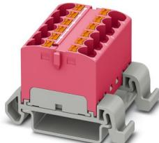
Distribution block, Block with horizontal alignment, nom. voltage: 800 V, nominal current: 32 A, number of connections: 12, connection method: Push-in connection, cross section: 0.2 mm<sup>2</sup> - 6 mm<sup>2</sup>, mounting type: NS 35/7,5, NS 35/15, color: pink
