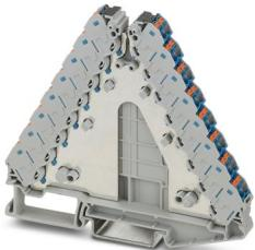
Potential distributors, nom. voltage: 250 V, nominal current: 17.5 A, connection method: Push-in connection, 1st, 2nd, 3rd, 4th, 5th, 6th, 7th and 8th level, Rated cross section: 1.5 mm<sup>2</sup>, cross section: 0.14 mm<sup>2</sup> - 2.5 mm<sup>2</sup>, mounting: NS 35/7,5, NS 35/15, color: gray, color of connection elements: blue
