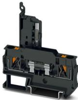
Fuse modular terminal block, fuse type: Glass / ceramics / ..., fuse type: G / 5 x 20, nom. voltage: 500 V, nominal current: 6.3 A, connection method: Push-in connection, 1 level, Rated cross section: 1 mm<sup>2</sup>, cross section: 0.2 mm<sup>2</sup>- 6 mm<sup>2</sup>, mounting type: NS 35/7,5, NS 35/15, color: black
