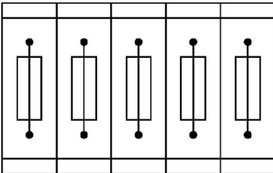
Fuse terminal blocks in interconnected arrangement,
