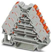
Marshalling panel, nom. voltage: 250 V, nominal current: 10 A, connection method: Push-in connection, 1st, 2nd, 3rd and 4th level, Rated cross section: 1.5 mm<sup>2</sup>, cross section: 0.14 mm<sup>2</sup> - 2.5 mm<sup>2</sup>, mounting: NS 35/7,5, NS 35/15, color: gray, color of connection elements: red
