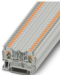
Feed-through terminal block, nom. voltage: 400 V, nominal current: 24 A, number of connections: 2, connection method: Push-in connection, Rated cross section: 2.5 mm<sup>2</sup>, cross section: 0.14 mm<sup>2</sup> - 4 mm<sup>2</sup>, mounting type: NS 35/7,5, NS 35/15, color: gray
