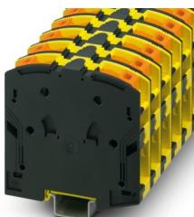
High-current terminal block, nom. voltage: 1000 V, nominal current: 232 A, number of connections: 2, number of positions: 1, connection method: PowerTurn connection, cross section: 25 mm<sup>2</sup> - 95 mm<sup>2</sup>, mounting type: NS 35/15, color: black/yellow
