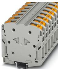
High-current terminal block, nom. voltage: 1000 V, nominal current: 232 A, number of connections: 2, number of positions: 1, connection method: PowerTurn connection, cross section: 25 mm<sup>2</sup> - 95 mm<sup>2</sup>, mounting type: NS 35/15, color: gray
