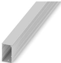
Cable duct for installation and mounting in control cabinets, gray, comprising upper part and mounting base, width: 60 mm, height: 100 mm, length: 2000 mm
