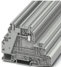
Multi-level terminal block, nom. voltage: 500 V, nominal current: 32 A, number of connections: 2, connection method: Screw connection, Rated cross section: 4 mm<sup>2</sup>, cross section: 0.14 mm<sup>2</sup> - 6 mm<sup>2</sup>, Screw connection, Rated cross section: 4 mm<sup>2</sup>, cross section: 0.14 mm<sup>2</sup> - 6 mm<sup>2</sup>, mounting type: NS 35/7,5, NS 35/15, color: gray
