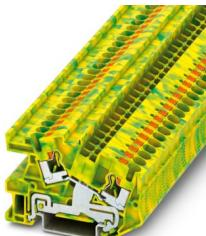
Installation protective conductor terminal block, Push-in connection, 1 level, Rated cross section: 4 mm<sup>2</sup>, cross section: 0.2 mm<sup>2</sup> - 6 mm<sup>2</sup>, mounting type: NS 35/7,5, NS 35/15, color: green-yellow
