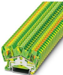
Protective conductor terminal block, number of connections: 2, connection method: Push-in connection, 1 level, cross section: 0.2 mm<sup>2</sup> - 6 mm<sup>2</sup>, mounting type: NS 35/7,5, NS 35/15, color: green-yellow
