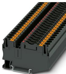
Fuse modular terminal block, fuse type: Blade, fuse type: Type C / max. 2.2 W, nom. voltage: 48 V, nominal current: 25 A, connection method: Push-in connection, Rated cross section: 6 mm<sup>2</sup>, cross section: 0.5 mm<sup>2</sup> - 10 mm<sup>2</sup>, mounting type: NS 35/7,5, NS 35/15, color: black
