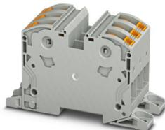
High-current terminal block, Blocked, nom. voltage: 1000 V, nominal current: 125 A, number of connections: 6, number of positions: 3, connection method: PowerTurn connection, Rated cross section: 35 mm<sup>2</sup>, cross section: 2.5 mm<sup>2</sup> - 35 mm<sup>2</sup>, mounting type: direct screw connection, color: gray
