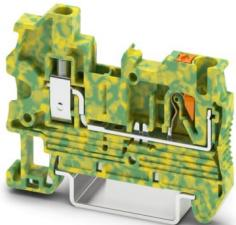
Protective conductor terminal block, connection method: Push-in connection, Rated cross section: 2.5 mm<sup>2</sup>, cross section: 0.14 mm<sup>2</sup> - 4 mm<sup>2</sup>, connection method: Screw connection, Rated cross section: 2.5 mm<sup>2</sup>, cross section: 0.14 mm<sup>2</sup> - 4 mm<sup>2</sup>, mounting: NS 35/7,5, NS 35/15, color: green-yellow
