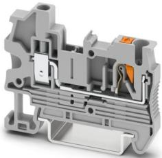
Feed-through terminal block, nom. voltage: 800 V, nominal current: 24 A, connection method: Push-in connection, Rated cross section: 2.5 mm<sup>2</sup>, cross section: 0.14 mm<sup>2</sup> - 4 mm<sup>2</sup>, connection method: Screw connection, Rated cross section: 2.5 mm<sup>2</sup>, cross section: 0.14 mm<sup>2</sup> - 4 mm<sup>2</sup>, mounting: NS 35/7,5, NS 35/15, color: gray
