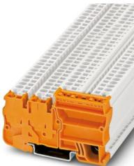
Power terminal block, nom. voltage: 250 V, nominal current: 30 A, number of connections: 2, connection method: Spring-cage connection, Rated cross section: 2.5 mm<sup>2</sup>, cross section: 0.08 mm<sup>2</sup> - 4 mm<sup>2</sup>, mounting type: NS 35/7,5, NS 35/15, color: orange
