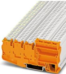
Installation protective conductor terminal block, nom. voltage: 250 V, nominal current: 30 A, number of connections: 5, connection method: Spring-cage connection, Rated cross section: 2.5 mm<sup>2</sup>, cross section: 0.08 mm<sup>2</sup> - 4 mm<sup>2</sup>, mounting type: NS 35/7,5, NS 35/15, color: orange
