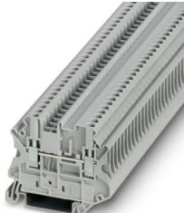
Feed-through terminal block, With test socket screws for insertion of test plugs, nom. voltage: 630 V, nominal current: 24 A, number of connections: 2, connection method: Screw connection, Rated cross section: 2.5 mm<sup>2</sup>, cross section: 0.14 mm<sup>2</sup> - 4 mm<sup>2</sup>, mounting type: NS 35/7,5, NS 35/15, color: gray
