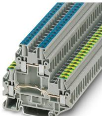
Feed-through terminal block, nom. voltage: 800 V, nominal current: 30 A, number of connections: 4, connection method: Screw connection, Rated cross section: 4 mm<sup>2</sup>, cross section: 0.14 mm<sup>2</sup> - 6 mm<sup>2</sup>, mounting type: NS 35/7,5, NS 35/15, color: gray
