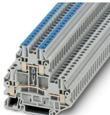
Feed-through terminal block, nom. voltage: 800 V, nominal current: 30 A, connection method: Screw connection, Rated cross section: 4 mm<sup>2</sup>, cross section: 0.14 mm<sup>2</sup> - 6 mm<sup>2</sup>, mounting type: NS 35/7,5, NS 35/15, color: gray
