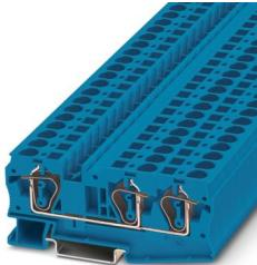
Feed-through terminal block, nom. voltage: 1000 V, nominal current: 41 A, number of connections: 3, connection method: Spring-cage connection, Rated cross section: 6 mm<sup>2</sup>, cross section: 0.2 mm<sup>2</sup> - 10 mm<sup>2</sup>, mounting type: NS 35/7,5, NS 35/15, color: blue
