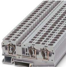
Feed-through terminal block, nom. voltage: 1000 V, nominal current: 41 A, number of connections: 3, connection method: Spring-cage connection, Rated cross section: 6 mm<sup>2</sup>, cross section: 0.2 mm<sup>2</sup> - 10 mm<sup>2</sup>, mounting type: NS 35/7,5, NS 35/15, color: gray
