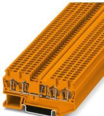
Component terminal block, with integrated diode, nom. voltage: 800 V, nominal current: 0.5 A, connection method: Spring-cage connection, Rated cross section: 1 mm<sup>2</sup>, cross section: 0.08 mm<sup>2</sup> - 4 mm<sup>2</sup>, mounting: NS 35/7,5, NS 35/15, color: orange
