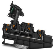
Fuse modular terminal block, fuse type: Glass / ceramics / ..., fuse type: G / 5 x 20, nom. voltage: 500 V, nominal current: 28 A, connection method: Push-in connection, Rated cross section: 4 mm<sup>2</sup>, cross section: 0.2 mm<sup>2</sup>- 6 mm<sup>2</sup>, connection method: Push-in connection, Rated cross section: 4 mm<sup>2</sup>, cross section: 0.2 mm<sup>2</sup>- 6 mm<sup>2</sup>, mounting type: NS 35/7,5, NS 35/15, color: black
