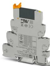
PLC-INTERFACE, consisting of PLC-BSC.../21 basic terminal block with screw connection and plug-in miniature solid-state relay, for mounting on NS 35/7,5, 1 N/O contact, input: 125 V DC, output: 3 - 48 V DC/100 mA
