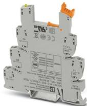
6.2 mm PLC basic terminal block for input functions with screw connection, without relay or solid-state relay, for mounting on NS 35/7.5 DIN rail, with sensor supply voltage distribution (BB), 1 N/O contact, input voltage: 230 V AC/DC
