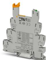
6.2 mm PLC basic terminal block with screw connection, without relay or solid-state relay, for mounting on DIN rail NS 35/7,5, 1 changeover contact, input voltage 120 V AC/DC
