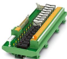
VARIOFACE output module, with plug-in bases for 16 miniature relays, 1 changeover contact each, for 24 V DC, with knife-disconnect terminal blocks in the output (without relays)
