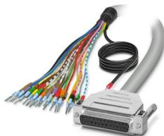
Assembled shielded round cable; connection 1: Single wires (25-position) (The wires are marked and fitted with ferrules. The braided shield is routed to a separate cable end.); connection 2: D-SUB socket strip (1x 25-position); cable length: 1 m
