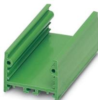
Press-drawn section housings, DIN rail mounting, Basic profile, profile width (internal): 22 mm, profile width (external): 24.8 mm, length: 1000 mm, Note: required profile length = PCB length - 3 mm
