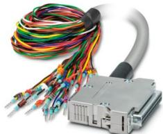
Assembled shielded round cable; connection 1: Twisted pair (37-position) (The wires are marked and fitted with ferrules); connection 2: D-SUB socket strip (1x 37-position); cable length: 3 m
