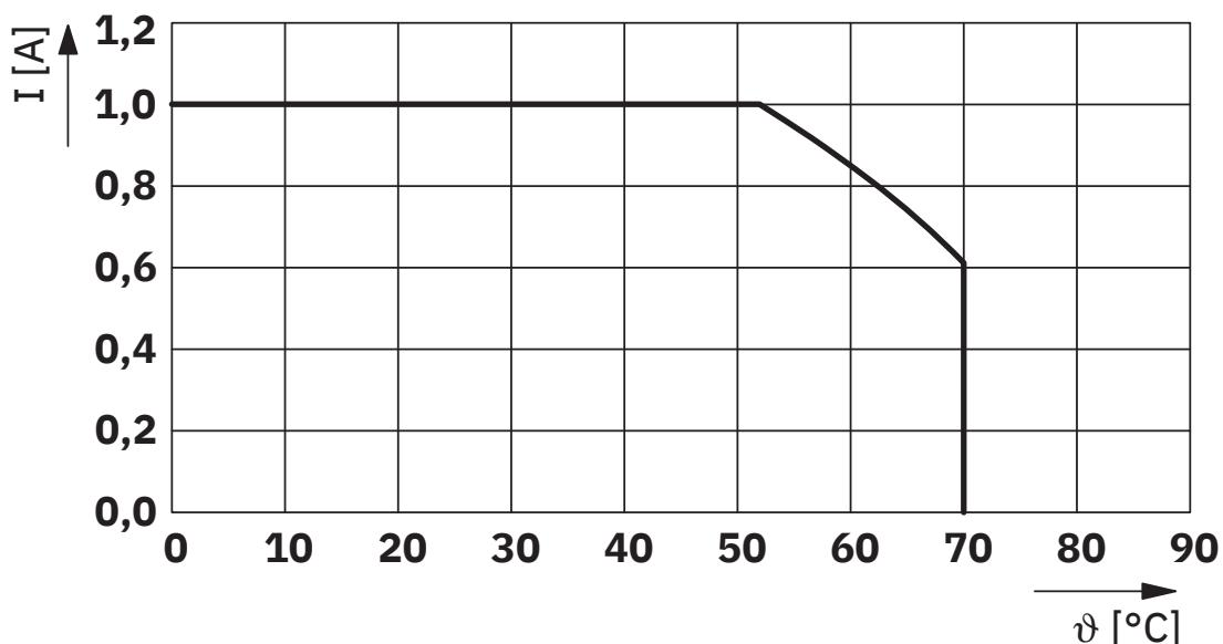
Maximum permissible current per path in uncoiled state
