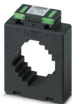
Window-type current transformer, 1000 A AC primary current; 1 A AC secondary current; accuracy class 1; 2.5 VA rated power
