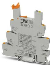
6.2 mm PLC basic terminal block with Push-in connection, without relay or solid-state relay, for mounting on DIN rail NS 35/7,5, 1 changeover contact, input voltage 230 V AC/DC
