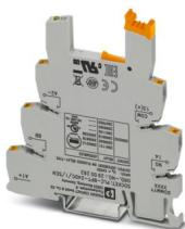
6.2 mm PLC basic terminal block for input functions with push-in connection, without relay or solid-state relay, for mounting on DIN rail NS 35/7,5, with sensor supply voltage distribution (BB), 1 N/O contact, input voltage 24 V DC
