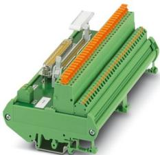
16-channel module for Honeywell C300 modules. The module is controlled by the control system via 37-pos. D-SUB or 50-pos. FLK. A spring-cage connection (1+, 1-,...16+,16-) with knife disconnection is provided in the field. Module width: 254 mm
