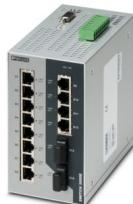
Managed Ethernet switch meets IEC 61850-3 and IEEE 1613 standards. Provides 12 RJ45 ports at 10/100 Mbps, two SC-D MM fiber optic ports and operating temperature of -40°C ... +70°C.
