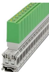
Plug-in relay interface for protection against interference on the control side, with soldered-in miniature switching relay, contacts (Au): small loads, 1 changeover contact, input voltage 24 V AC/DC
