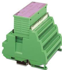
INTERBUS-ST digital input/output module, 8 inputs, 24 V DC, 8 outputs, 24 V DC, 2 A, IP20 protection, consisting of: Terminal part with spring-cage connection and module electronics, extended temperature range
