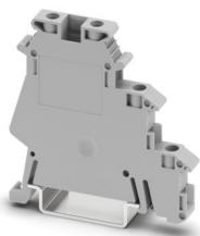
Initiator/actuator terminal block, nom. voltage: 250 V, nominal current: 24 A, connection method: Screw connection, 1st, 2nd and 3rd level, Rated cross section: 2.5 mm<sup>2</sup>, cross section: 0.2 mm<sup>2</sup> - 4 mm<sup>2</sup>, mounting type: NS 35/7,5, NS 35/15, color: gray
