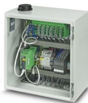
Measurement system for load characteristics and bending moments in rotor blades of wind turbine generators. Proactive rotor blade monitoring, early detection of damage, and optimized load control. Reliable in harsh ambient conditions and suitable for remote service.
