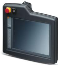
Mobile panel, 26.4 cm / 10.4"-TFT display (Resistive industrial touch screen), 800 x 600 pixel(s) (SVGA), 65536 colors, Xscale® PXA320, 806 MHz, 1x USB Host 1.1, 1 x Ethernet (10/100 Mbps), RJ45, Windows® CE 5.0, NetCap / Portico, without bus system.
