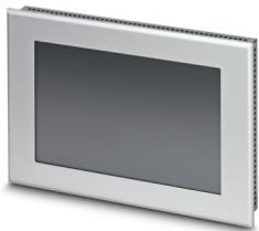
Touch panel, 22.9 cm / 9"-TFT display (analog resistive (polyester)), 800 x 480 pixel(s) (WVGA), 262144 colors, Xscale® PXA320, 806 MHz, 2x USB host 1.1, 1 x Ethernet (10/100 Mbps), RJ45, Windows® CE 5.0, TSvisRT, CAN.
