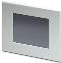
Rugged-Touch panel, 17.8 cm / 7"-TFT display (Analog resistive (GFG)), 800 x 480 pixel(s) (WVGA), 16.7 million colors, Arm® Cortex®-A8, 1000 MHz, 2x USB Host 2.0, 1 x Ethernet (10/100 Mbps), RJ45, Windows® Embedded Compact 7, Open platform, without bus system.
