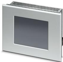
Touch panel, 14.5 cm / 5.7"-TFT display (analog resistive (polyester)), 320 x 240 pixel(s) (QVGA), 262144 colors, Xscale® PXA320, 806 MHz, 2x USB host 1.1, 1 x Ethernet (10/100 Mbps), RJ45, Windows® CE 6.0, Movicon™, without bus system.
