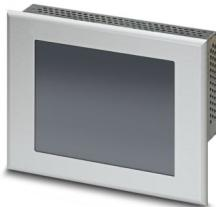
Touch panel, 14.5 cm / 5.7"-FSTN display (analog resistive (polyester)), 320 x 240 pixel(s) (QVGA), 256 grayscales, Arm9™, 200 MHz, 2x USB Host 2.0, 1 x Ethernet (10/100 Mbps), RJ45, Windows® CE 6.0, Open platform, without bus system.
