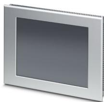
Touch panel, 26.4 cm / 10.4"-TFT display (analog resistive (polyester)), 800 x 600 pixel(s) (SVGA), 262144 colors, Xscale® PXA320, 806 MHz, 2x USB host 1.1, 1 x Ethernet (10/100 Mbps), RJ45, Windows® CE 5.0, TSvisRT, without bus system.
