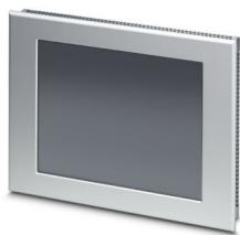
Touch panel, 26.4 cm / 10.4"-TFT display (analog resistive (polyester)), 640 x 480 pixel(s) (VGA), 65536 colors, Arm9™, 200 MHz, 2x USB Host 2.0, 1 x Ethernet (10/100 Mbps), RJ45, Windows® CE 5.0, TSvisRT, without bus system.
